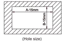
Step 2: 10 Draw the cutting line and cut the install hole;
