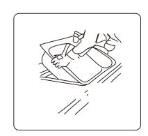
Step 4: ① Check again the position of the sink on the counter and glue appropriate glass cement at the edge of the sink.
